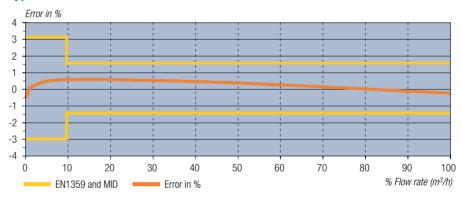
Every meter undergoes a 100% inspection for function, accuracy and safety. All meters are EN1359 compliant and have DVGW approval.
